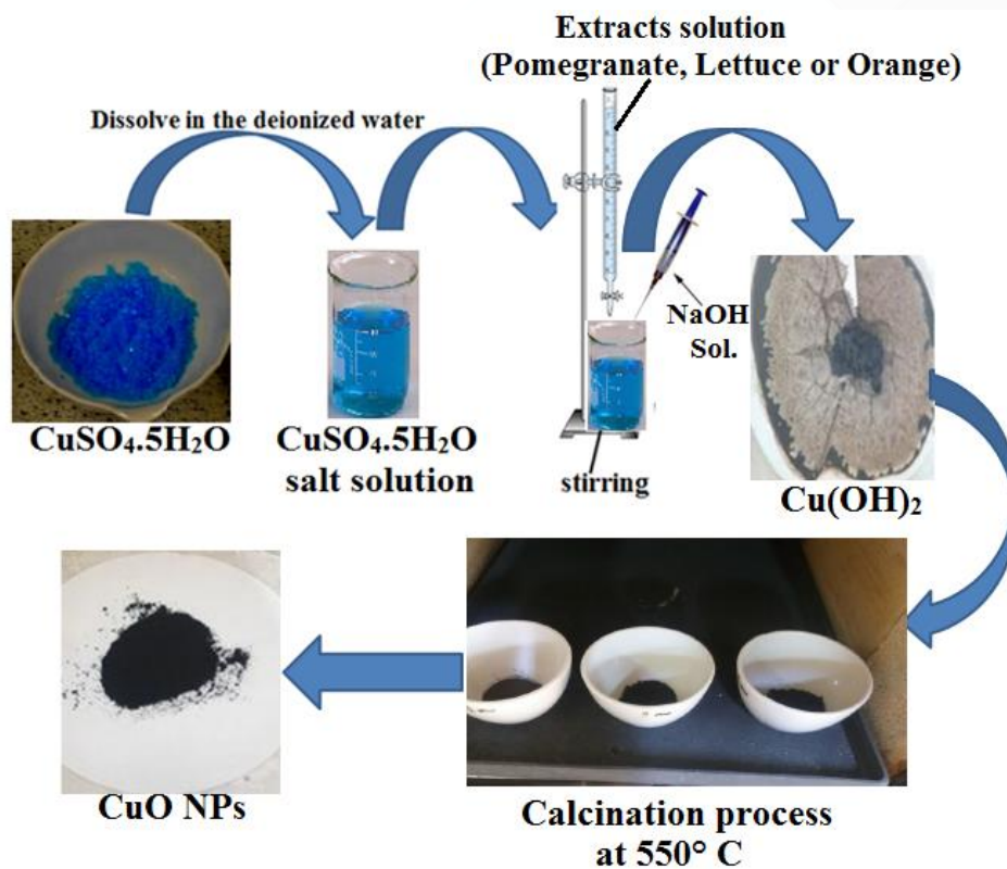
Scheme 1. Preparation of Copper oxide nanoparticles by Pomegranate, Lettuce or Orange leaves extract as a reduction factor with NaOH as precipitation agent
